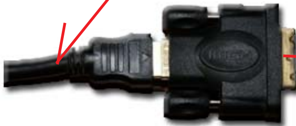
Video cable (HDMI) attached to the DVI adapter that will be plugged into the big screen.
