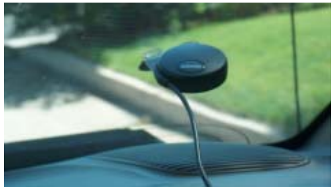
Place the Garmin GPS-18 sensor on the car dash or use the windshield suction cup mount. (This is mounted higher than necessary to make it more visible in this photo).
